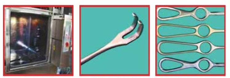
Titanium oxide discoloration occurs mostly on <u>reflective surfaces</u> over large surfaces, yellow-brown to blue-violet, sometimes with a shimmering appearance, in the wash chamber or over the entire surface of the instrument during machine-cleaning.
